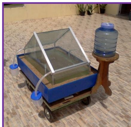
Gambar 3. Unit Destilasi Solar Heater
