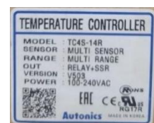
Gambar 16 Name Plate Termocontrol
