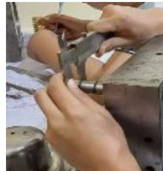
Gambar 3. Proses pengukuran part molding
