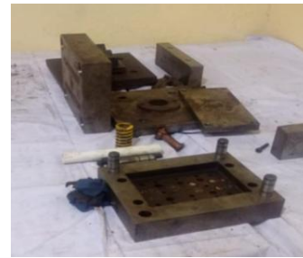
Gambar 2. Potongan part molding pallet seng
